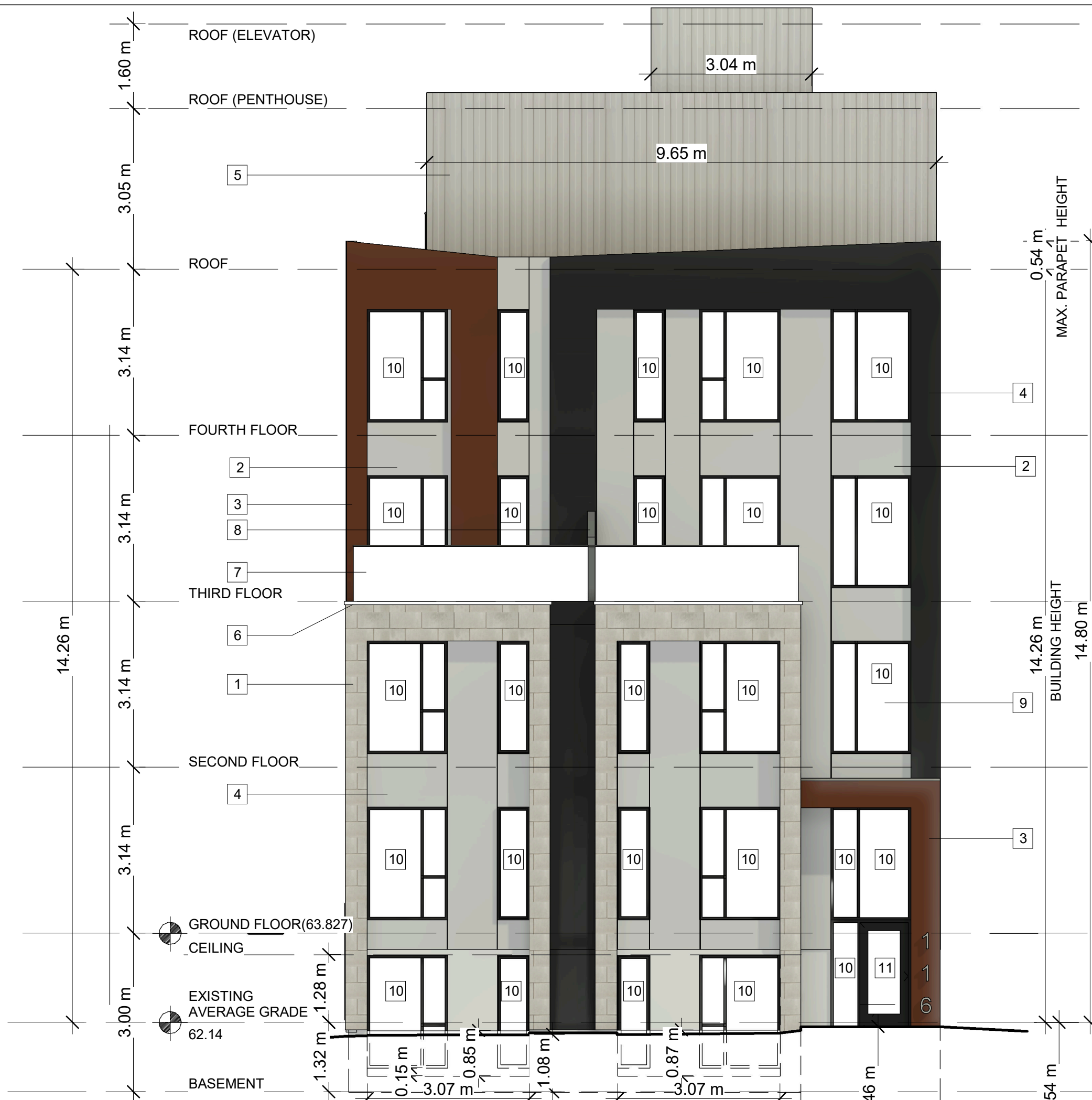
1 Front (East) Elevation 1 : 75
