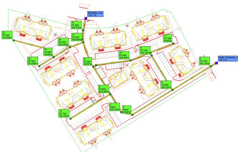
Figure 3.4 Minimum Pressures (psi) in Block 167 During PKHR Conditions after SUC Pressure Zone Reconfiguration
