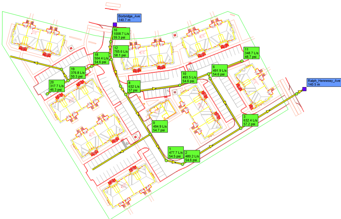
Figure 3.5 Available Fire Flows (L/s) in Block 167 During MXDY Conditions after SUC Pressure Zone Reconfiguration
