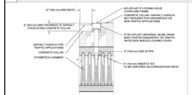
INSPECTION PORTS MAY BE CONNECTED THROUGH ANY CHAMBER CORRUGATION CREST.
