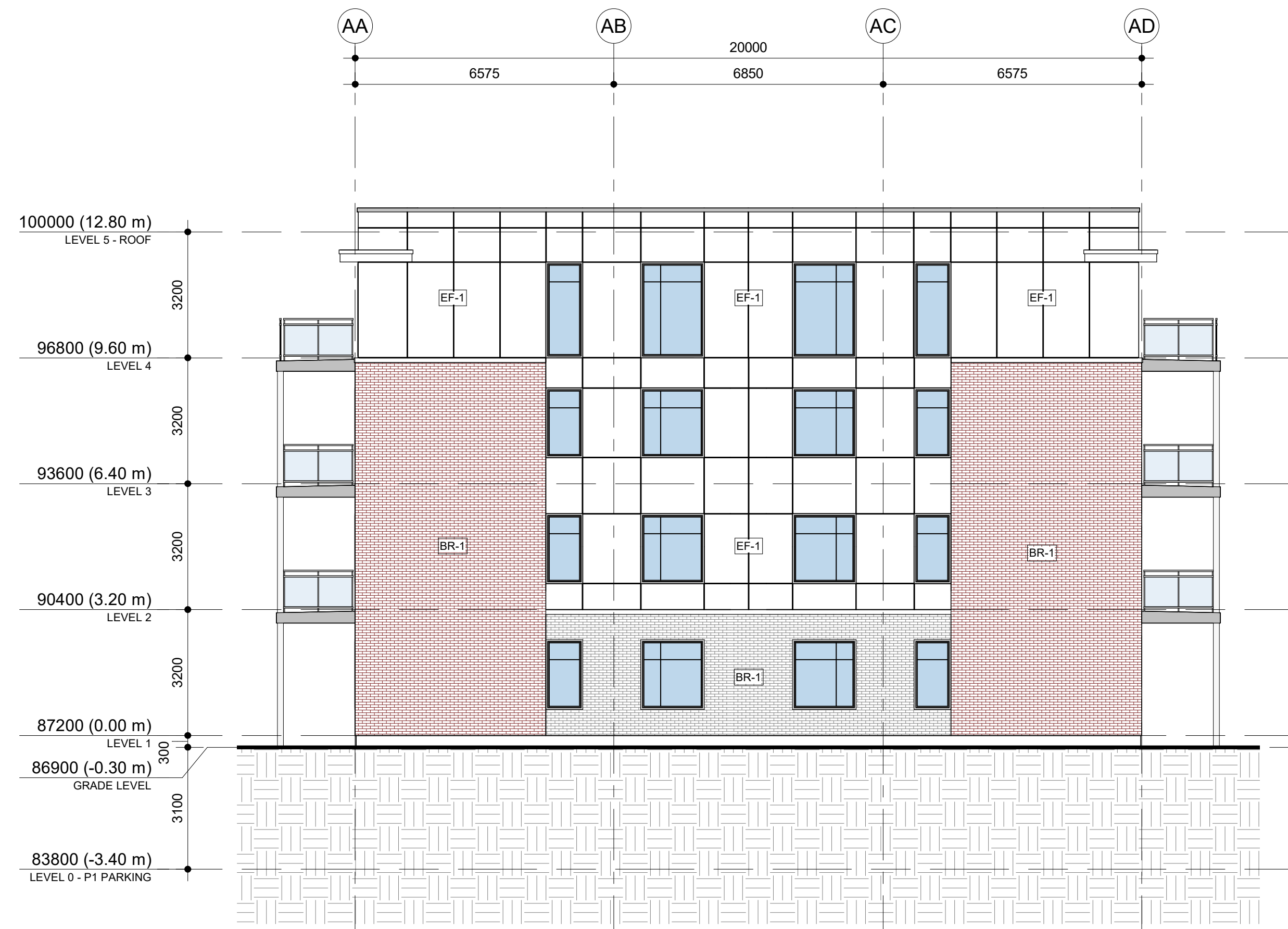
2 BUILDING A - SOUTH ELEVATION A201 1 : 100
