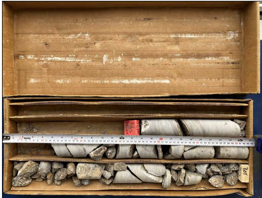
Photo 6: Photograph of RC 6 from BH 1-23 – Depth from 9.14 to 10.64 m – RQD = 68 % and REC = 89 %
