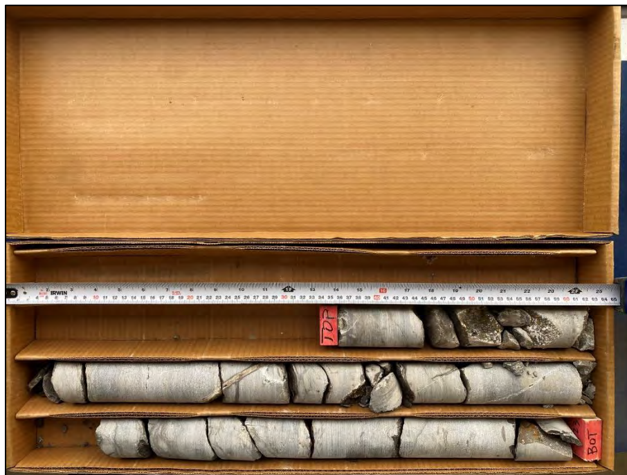
Photo 6: Photograph of RC 6 from BH 1-23 – Depth from 9.14 to 10.64 m – RQD = 68 % and REC = 89 %
