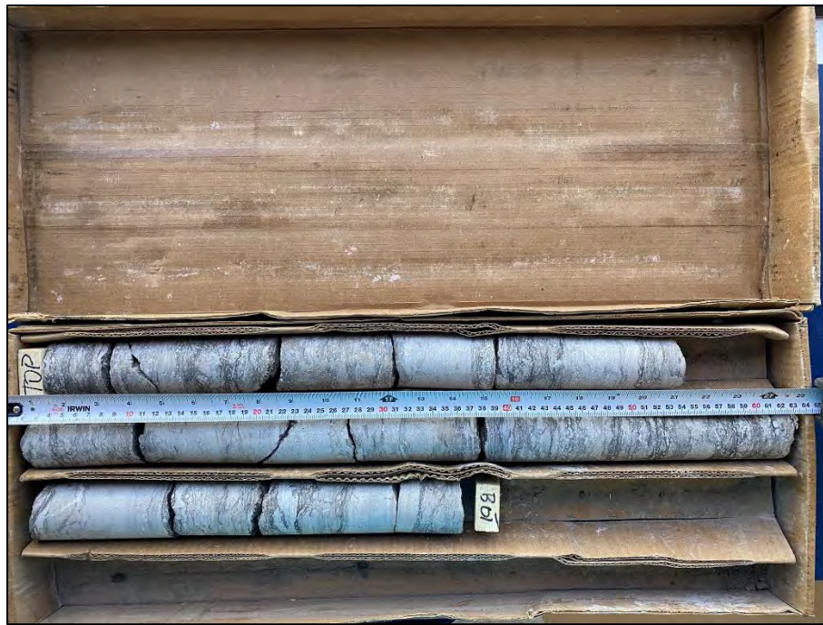
Photo 32: Photograph of RC 10 from BH 4-23 – Depth from 13.61 to 15.11 m – RQD = 100 % and REC = 100 %
