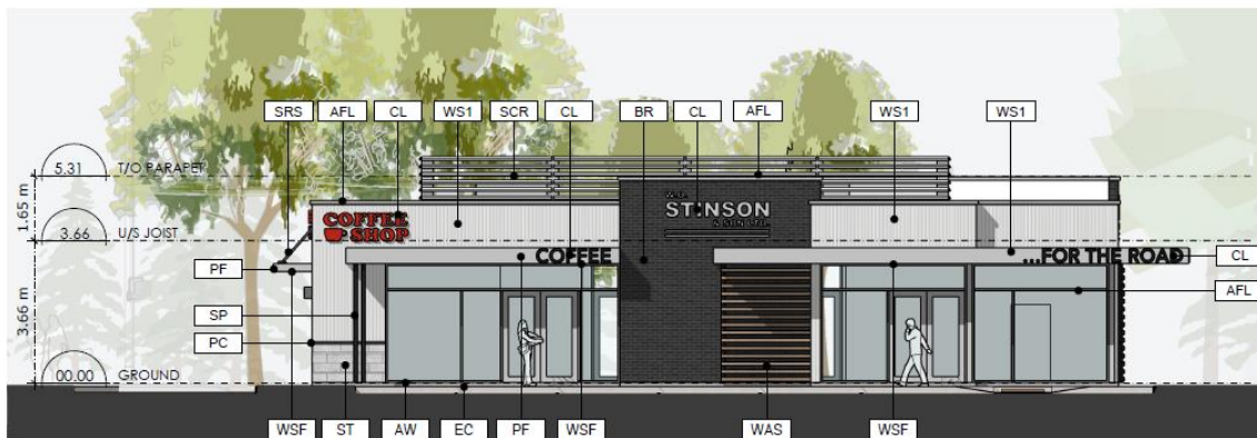
Figure 4. Excerpt of Concept Elevations – South and East (Hobin Architecture).
