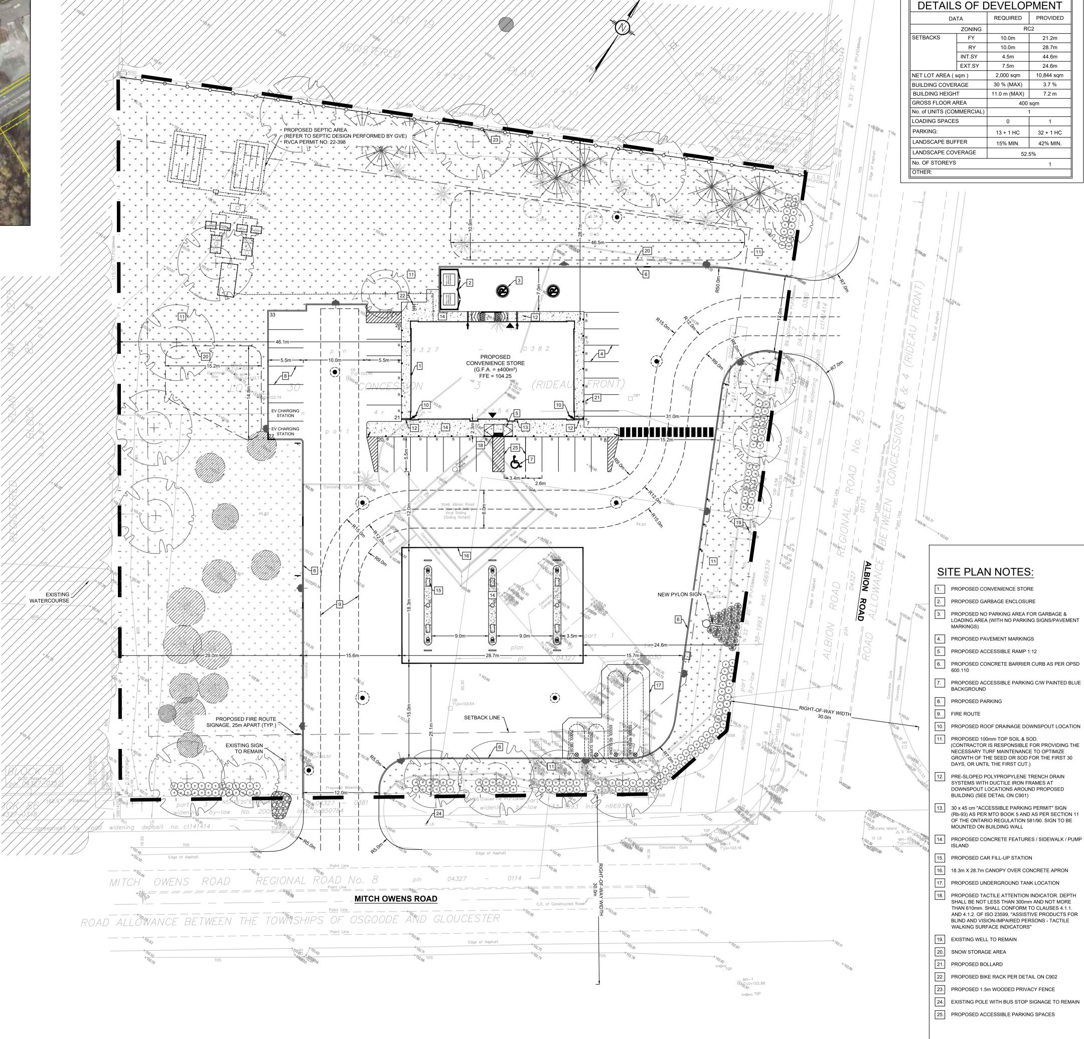
DETAILS OF DEVELOPMENT REQUIRED PROVIDED 10.0m 10.0m 28.7m 4.5m 7.5m 24.6m 2,000 sqm 10,844 sqm 30 % (MAX) 11.0 m (MAX) 7.2 m 400 sqm 13 + 1 HC 32 + 1 HC 15% MIN. 42% MIN. 52.5%
