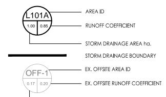
EX. OFFSITE STORM DRAINAGE AREA ha. EX. OFFSITE STORM DRAINAGE BOUNDARY
