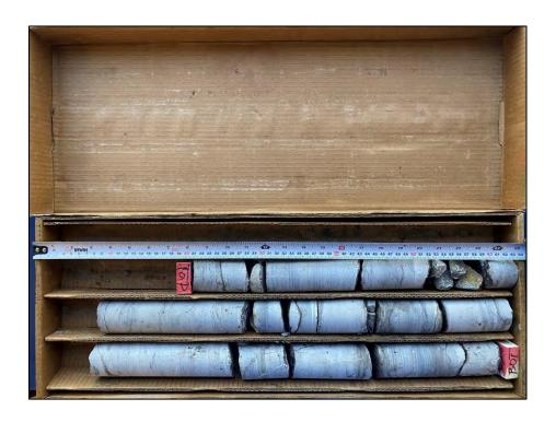
**Photo 14:** Photograph of RC 3 from BH 2-23 – Depth from 4.67 to 6.17 m – RQD = 73 % and REC = 100 %
