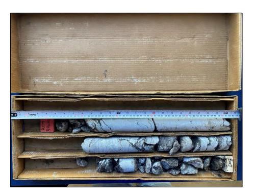
**Photo 21:** Photograph of RC 10 from BH 2-23 – Depth from 15.16 to 16.69 m – RQD = 37 % and REC = 80 %
