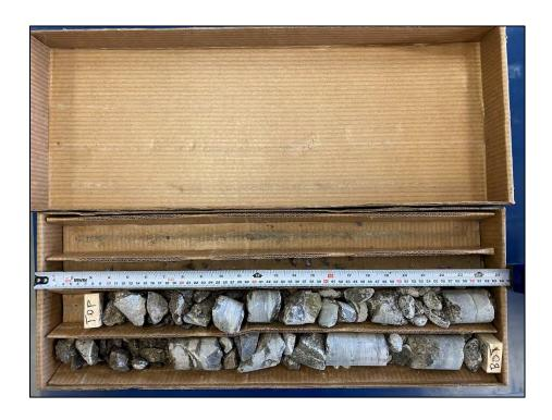
**Photo 10:** Photograph of RC 10 from BH 1-23 – Depth from 15.14 to 16.51 m – RQD = 59 % and REC = 100 %
