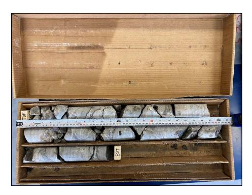
**Photo 43:** Photograph of RC 10 from BH 5-23 - Depth from 18.11 to 19.58 m - RQD = 50 % and REC = 100 %
