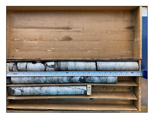
**Photo 34:** Photograph of RC 1 from BH 5-23 – Depth from 5.72 to 6.32 m – RQD = 0 % and REC = 100 %
