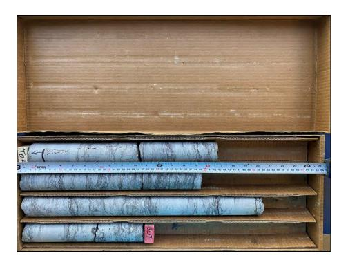
**Photo 33:** Photograph of RC 11 from BH 4-23 – Depth from 15.11 to 16.64 m – RQD = 83 % and REC = 100 %
