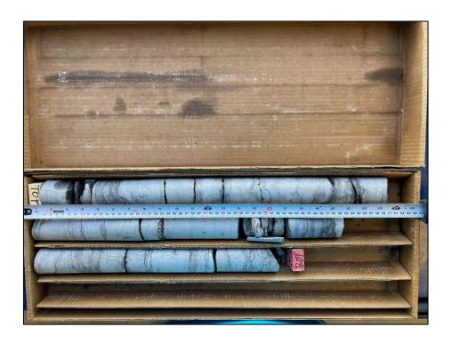
**Photo 28:** Photograph of RC 6 from BH 4-23 – Depth from 7.62 to 9.12 m – RQD = 97 % and REC = 100 %
