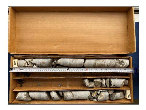
**Photo 8:** Photograph of RC 8 from BH 1-23 – Depth from 12.14 to 13.64 m – RQD = % and REC = 93 %
