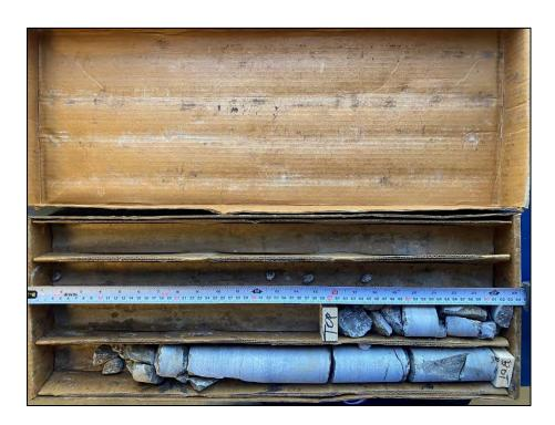
**Photo 13:** Photograph of RC 2 from BH 2-23 – Depth from 3.18 to 4.67 m – RQD = 76 % and REC = 100 %
