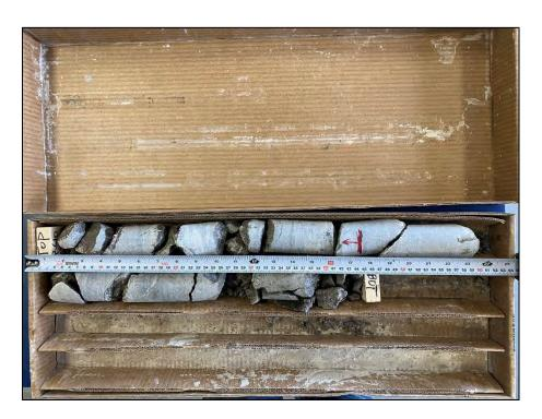
**Photo 11:** Photograph of RC 11 from BH 1-23 – Depth from 16.51 to 18.39 m – RQD = 53 % and REC = 100 %
