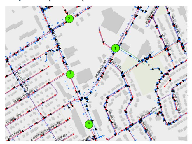
• Outlet #1 is the natural drainage point for this sanitary system, however the Parkwood Hills system was never designed for such a large domestic input at it's upstream end. When we add the 36 L/s flow to it, we get significant surcharge that reaches basement elevation and even the ground. See image below. This system does not work for 36 L/s or even 18 L/s.
