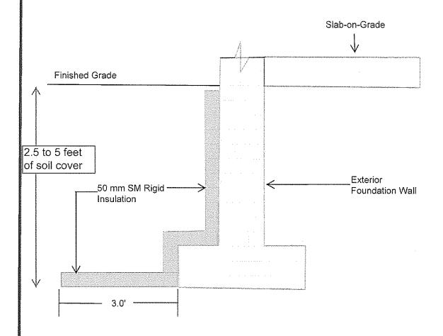
This detail applies where there is between 2.5 and 5 feet of soil cover above the underside of footing (USF) elevation. Where the soil cover is equal to, or greater than, 5 feet, the foundation insulation can be omitted.
