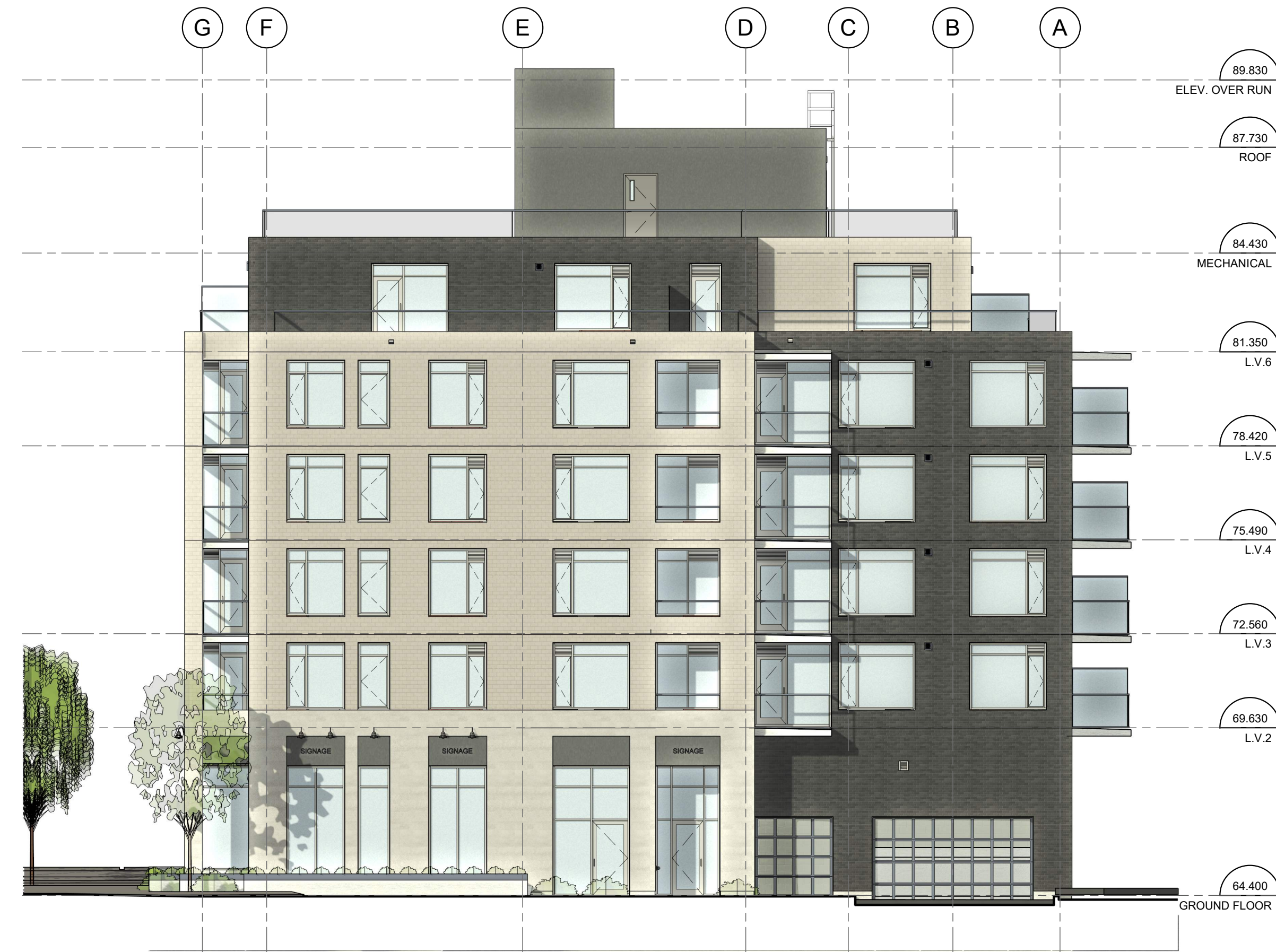
2 SOUTH ELEVATION - SPRINGHURST AVE D109 1 : 125
