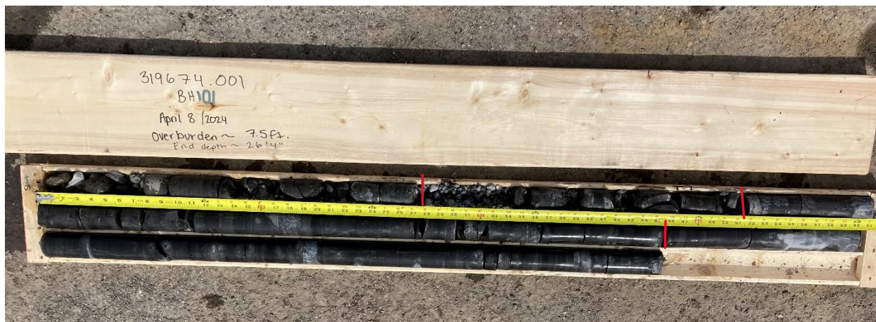
Photo 1 – Bedrock Core Borehole BH1, 2.3 to 8.1 mbgs, RC1, RC2, RC3 and RC4
