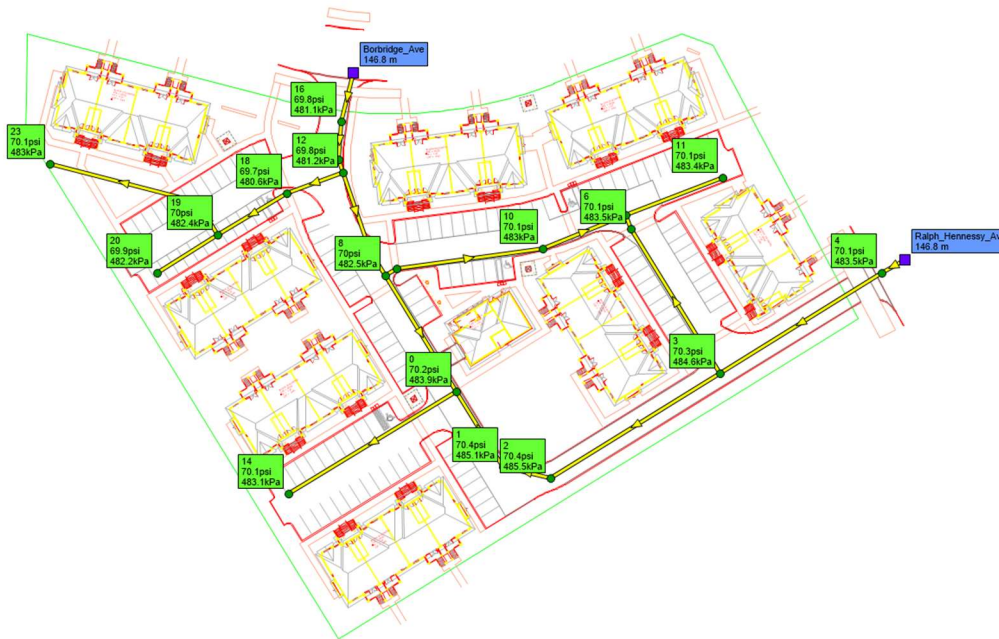
Figure 3.3 Maximum Pressures in Block 167 (during AVDY Conditions after SUC Pressure Zone Reconfiguration)
