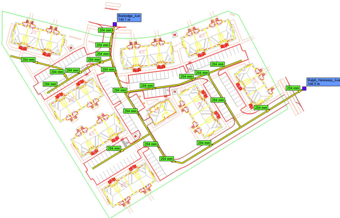
Figure 3.1 Proposed Watermain Layout and Pipe Diameters (mm)
