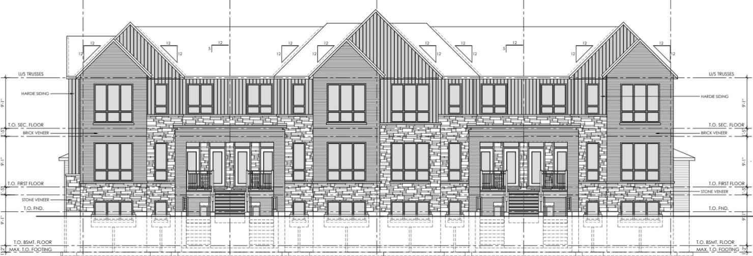
STREET END UNIT - ELEV. 'C' MID UNIT REV. - ELEV. 'C' MID UNIT - ELEV. 'C' END UNIT REV. - ELEV. 'C'
