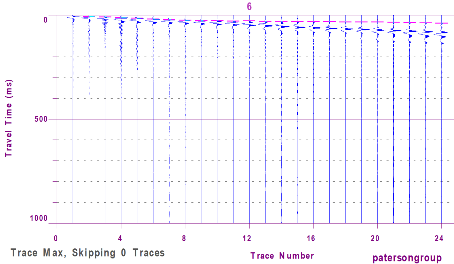
Figure 2 – Shear Wave Velocity Profile at Shot Location -3.5 m
