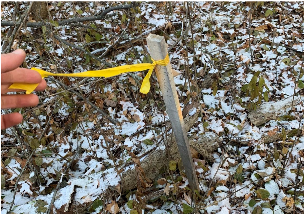
Photo 16: Stake indicating inferred proposed borehole location on-Site.
