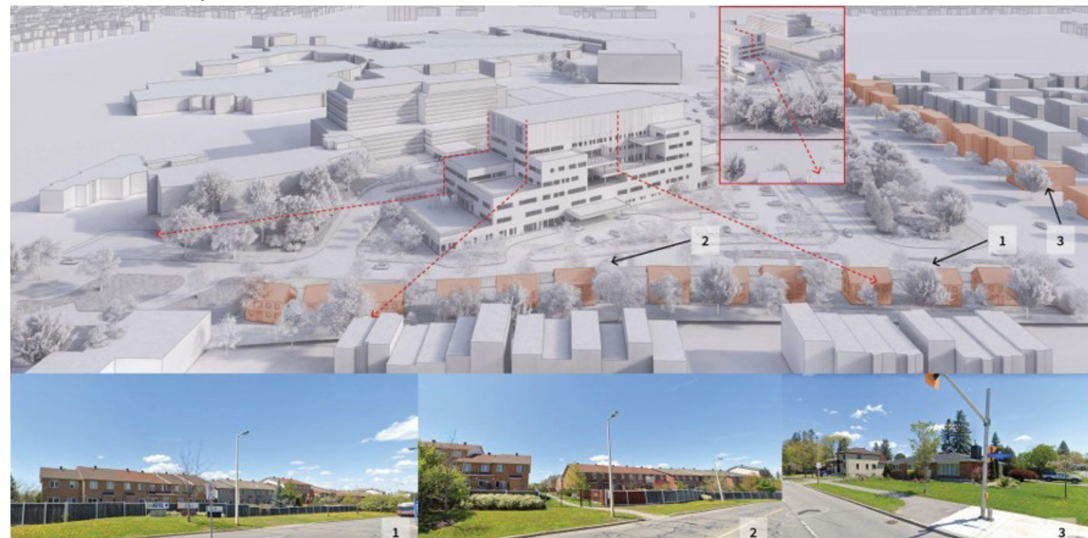
Massing Response to Context | Low massing steps down towards west, south and north to minimize impact on low residential context
