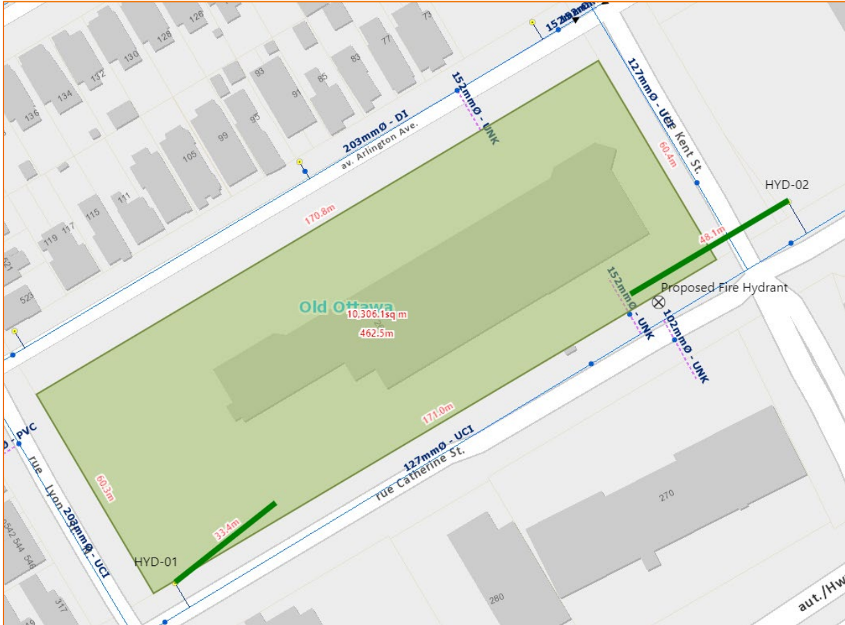
Figure 3.1: Fire Hydrant Coverage Sketch
