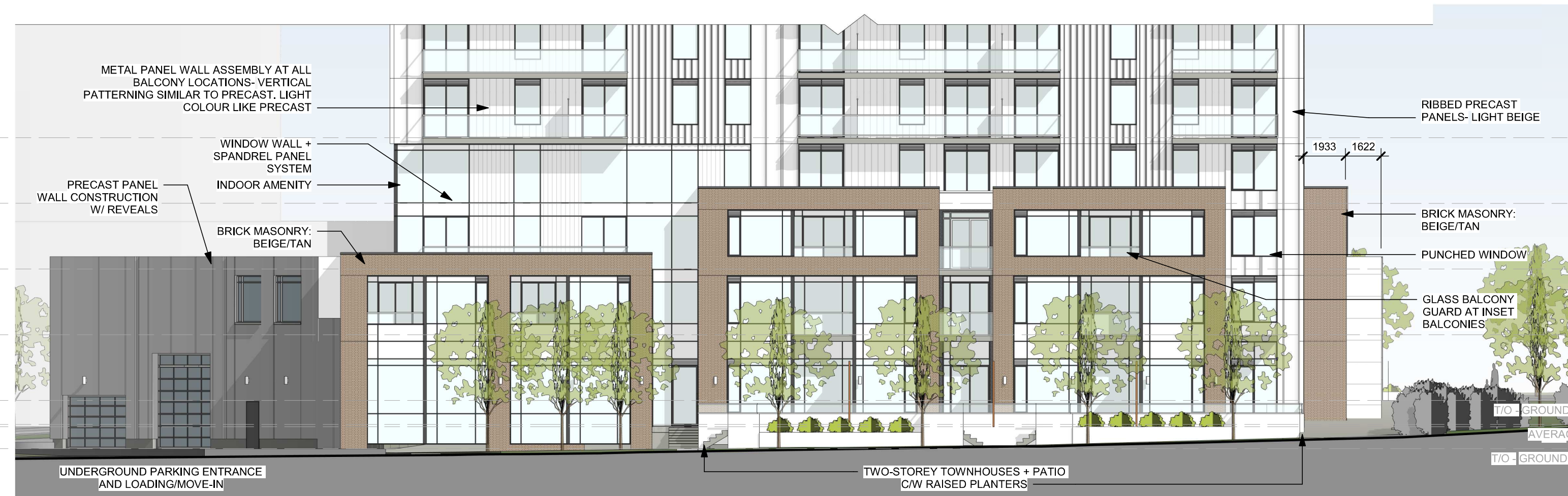
1 ENLARGED ELEVATION - WEST A-203 1:175
