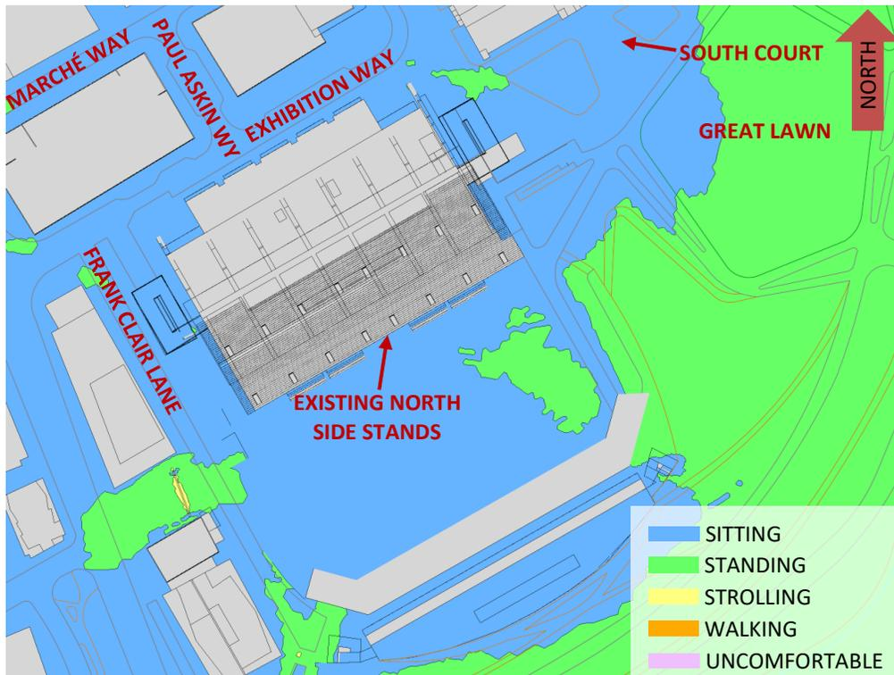
**FIGURE 3B: SPRING – WIND COMFORT, TD PLACE – EXISTING**
