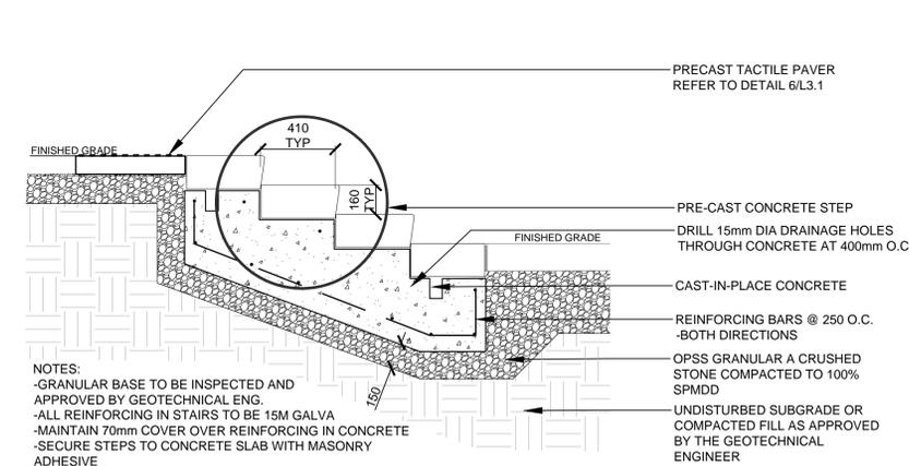
3 PRECAST CONCRETE STEPS ON C.I.P. FOOTING
