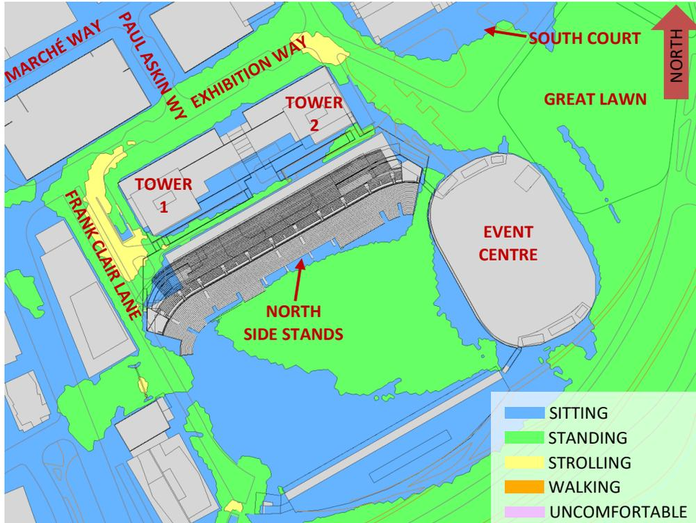
**FIGURE 3A: SPRING – WIND COMFORT, TD PLACE – PROPOSED**
