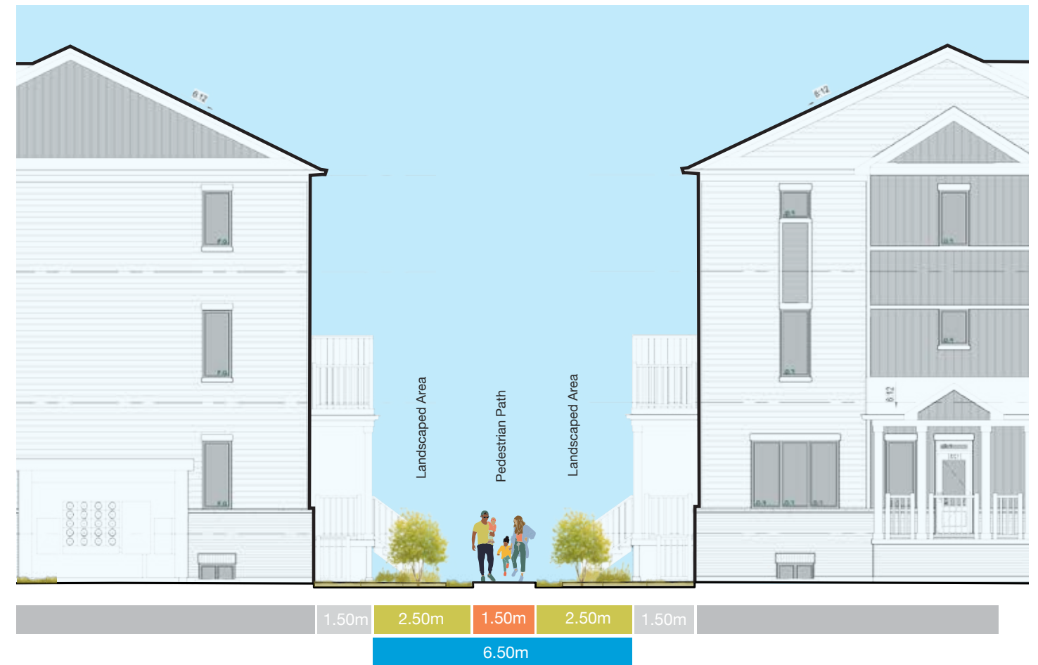
Figure 23 - Section C-C signified on Site Plan Conectivity
