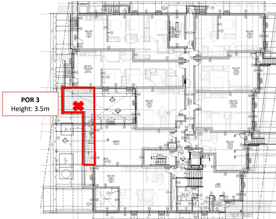
**Figure 4.5** – Floor Plan of the Level 1 patio Outdoor Living Area (POR3) of 10-20 Empress Ave. The space associated with the POR is outlined in red. The red 'X' denotes the receiver location used in STAMSON.
