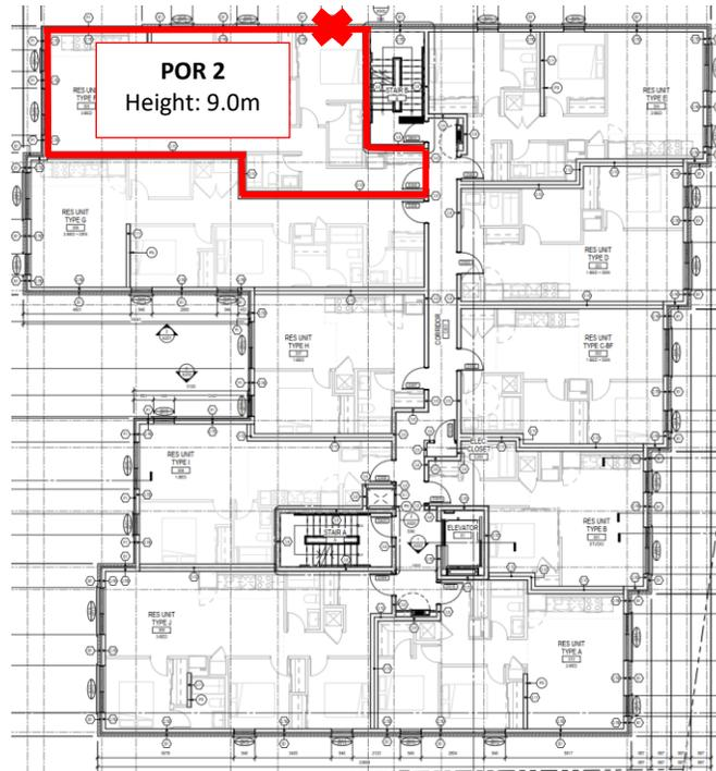
**Figure 4.4** – Floor Plan of 3<sup>rd</sup> floor (POR2) of 10-20 Empress Ave. The room associated with the POR is outlined in red. The red 'X' denotes the receiver location used in STAMSON.
