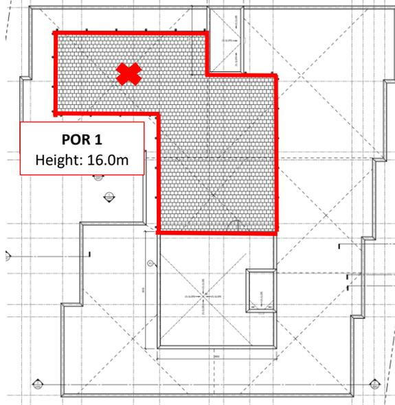
**Figure 4.3** – Floor Plan of the rooftop Outdoor Living Area (POR1) of 10-20 Empress Ave. The space associated with the POR is outlined in red. The red 'X' denotes the receiver location used in STAMSON.
