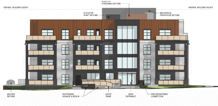
Figure 12.0 – South elevation (August 2024).
