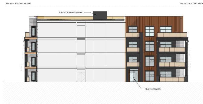
Figure 12.3 – North elevation/section showing rear entry condition (August 2024).
