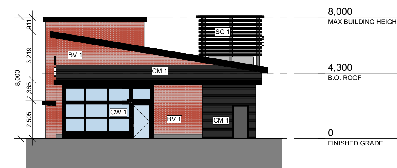
3 BUILDING F - WEST ELEVATION 1:150
