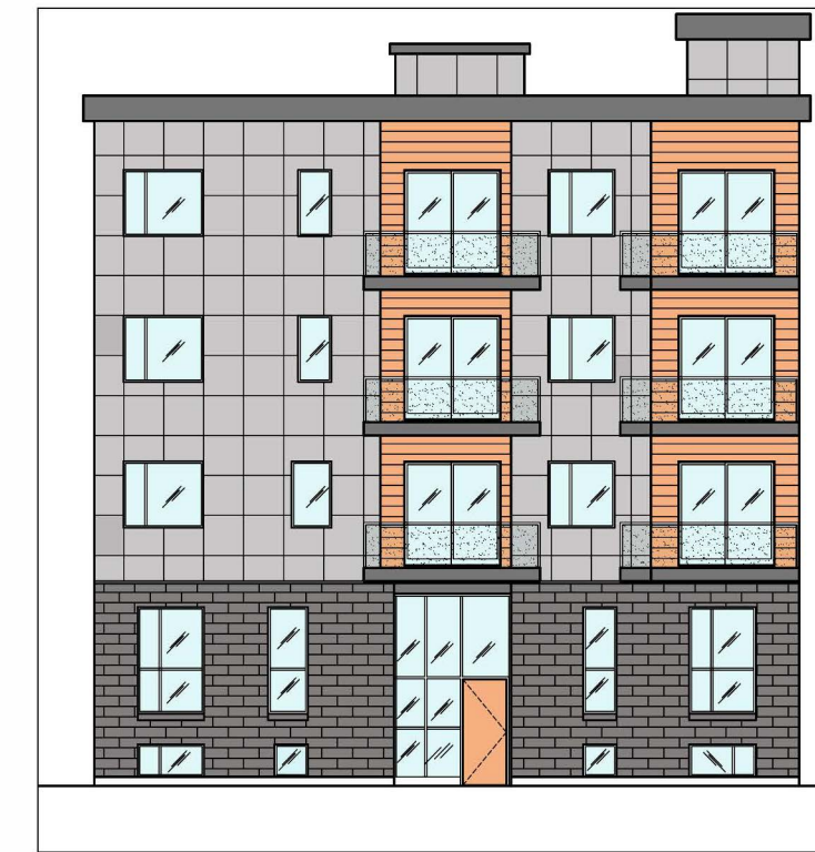
1 FRONT (NORTH) FACADE SCALE = 1/16" = 1'-0"
