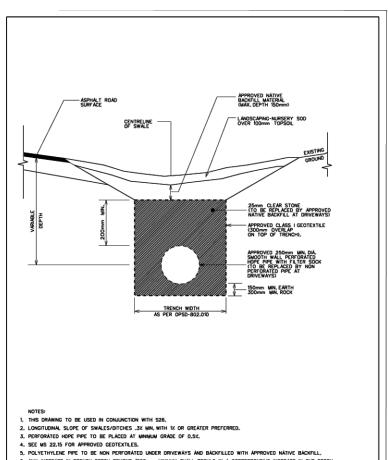
ANY INCREASE IN TRENCH DEPTH BEYOND 1000mm MINIMUM SHALL RESULT IN A CORRESPONDING INCREASE IN THE DEPTH OF 25mm CLEAR STONE ABOVE PERFORATED PIPE.
