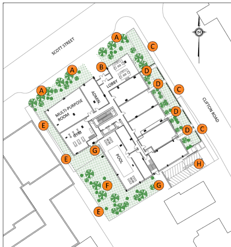
1950 SCOTT STREET – GRADE REFERENCE MARKER LOCATIONS
