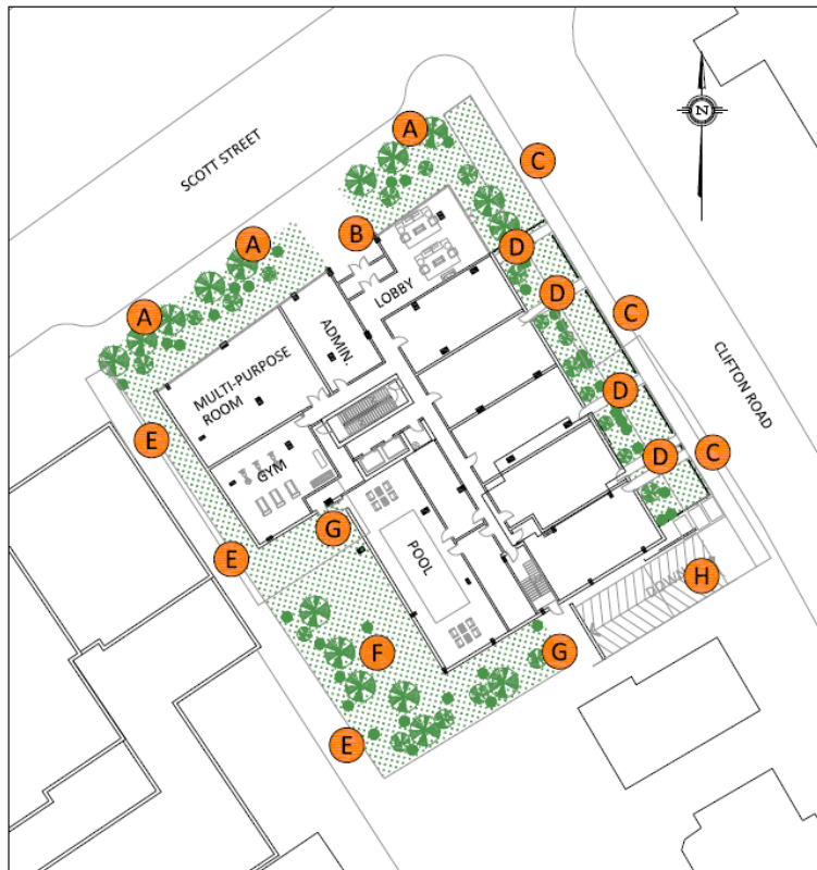
1950 SCOTT STREET – GRADE REFERENCE MARKER LOCATIONS
