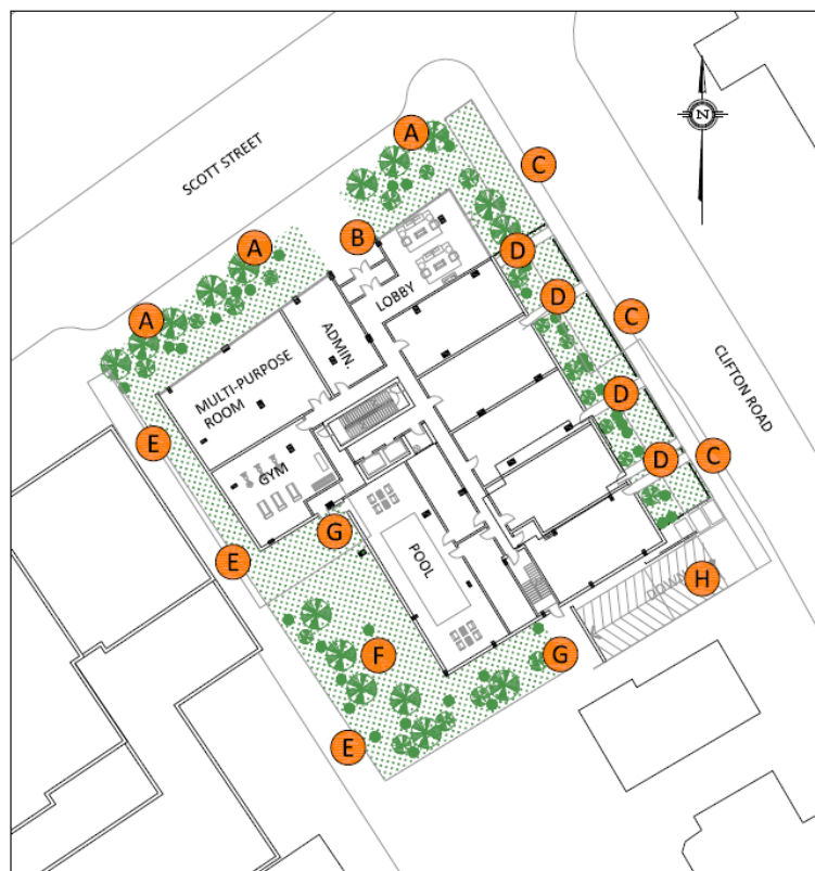
1950 SCOTT STREET – GRADE REFERENCE MARKER LOCATIONS
