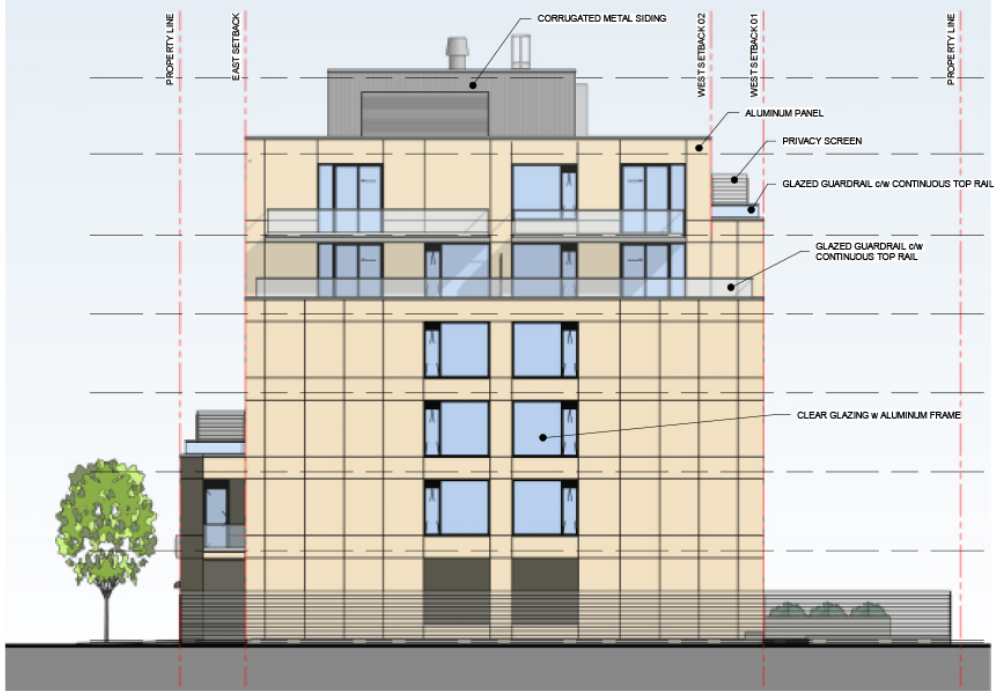
NEW NORTH ELEVATION
