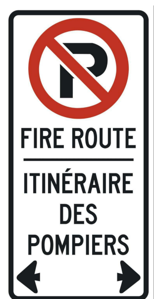
PROVIDE VERTICAL SIGNAGE AT 25 m SPACING MAXIMUM
