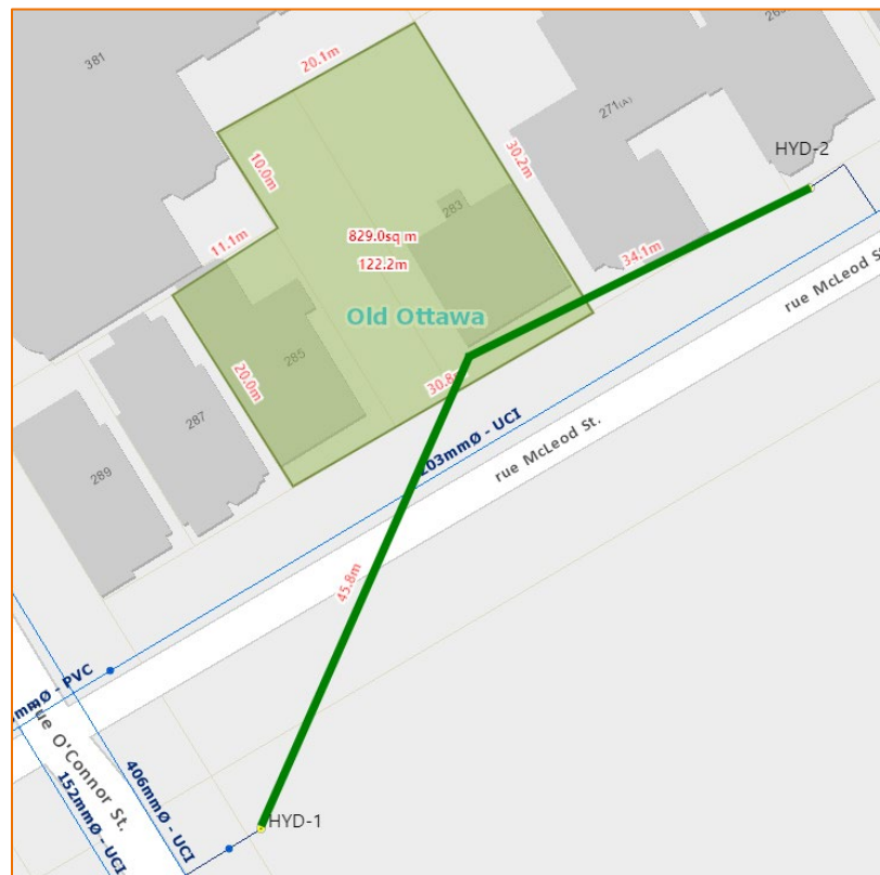
Figure 3.1: Existing Fire Hydrant Coverage Map
