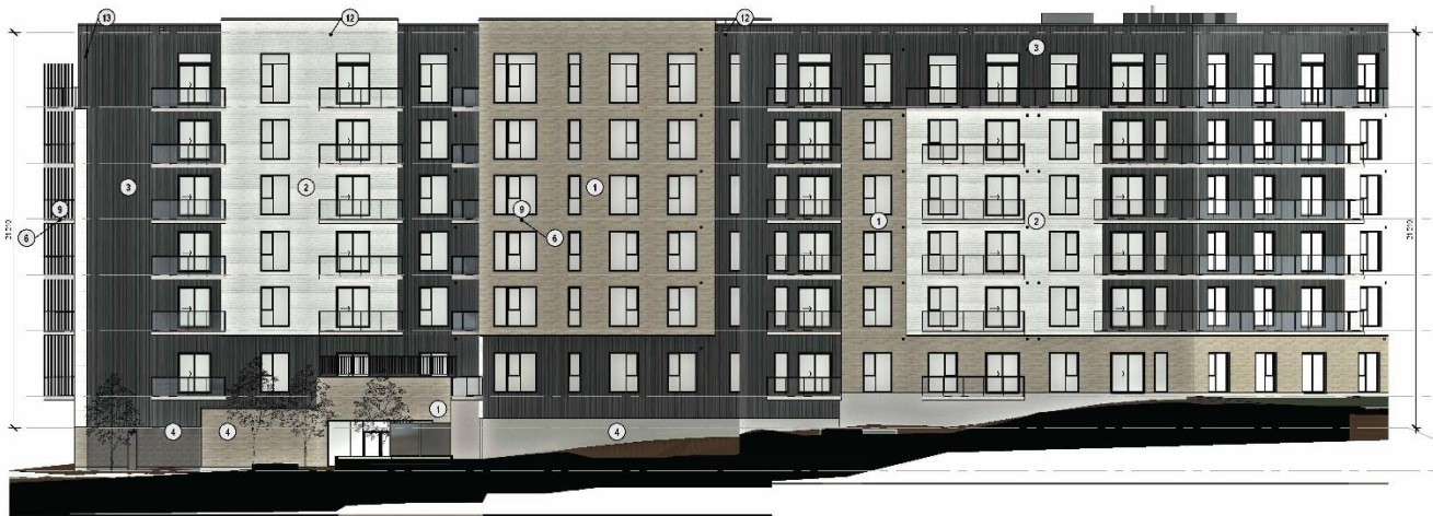
Figure 16: West and Southwest Elevation drawing of the proposed development, showing the change in grade from March Road (right) to Shirley's Brook (left)
