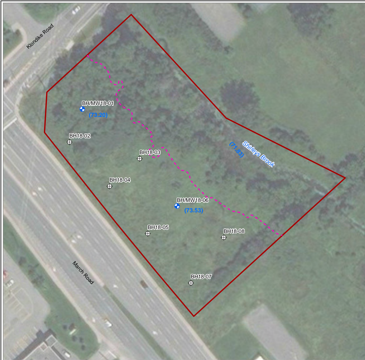
Figure A.5 Groundwater Elevation and Interpretted Flow Direction
