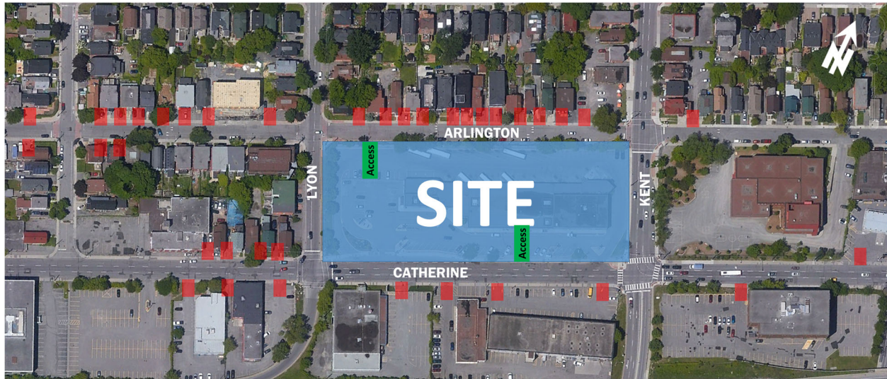
Figure 4: Adjacent Driveways within 200m of Site Access
