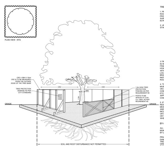
TREE PROTECTION REQUIREMENTS: PRIOR TO ANY WORK ACTIVITY WITHIN THE CRITICAL
