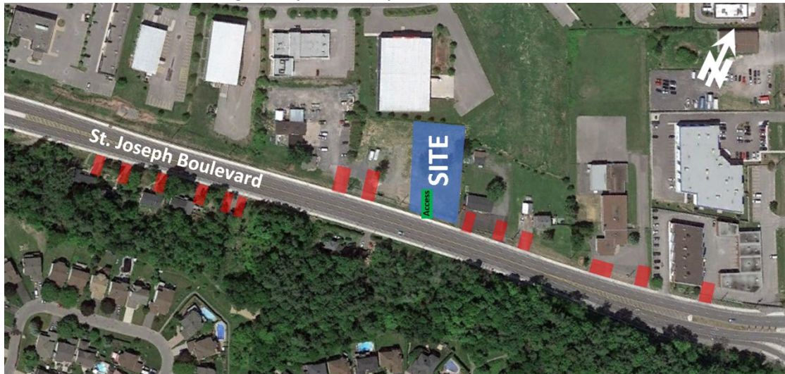
Figure 3: Adjacent Driveways within 200m of Site Access
