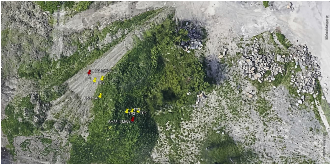
Figure 1. Infiltration Testing and Monitoring Well Locations
