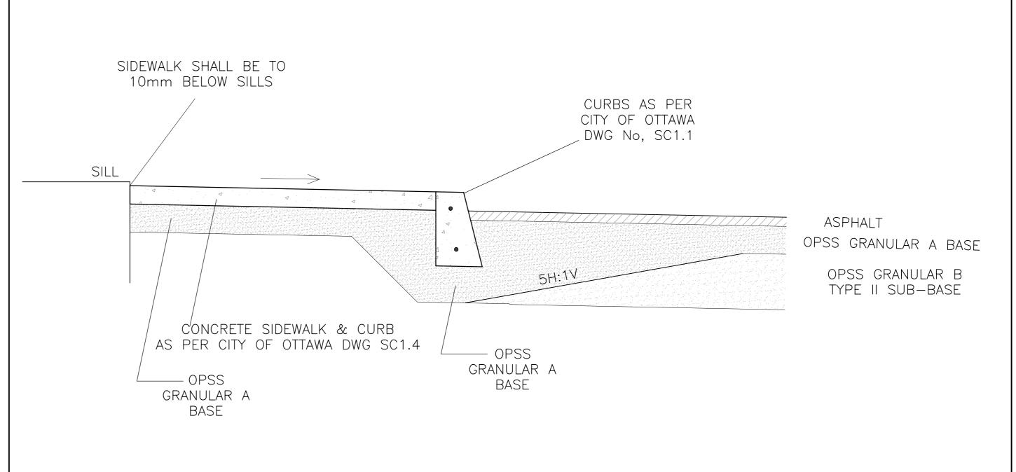
CONCRETE SIDEWALK / CURB / PAVEMENT SECTION
