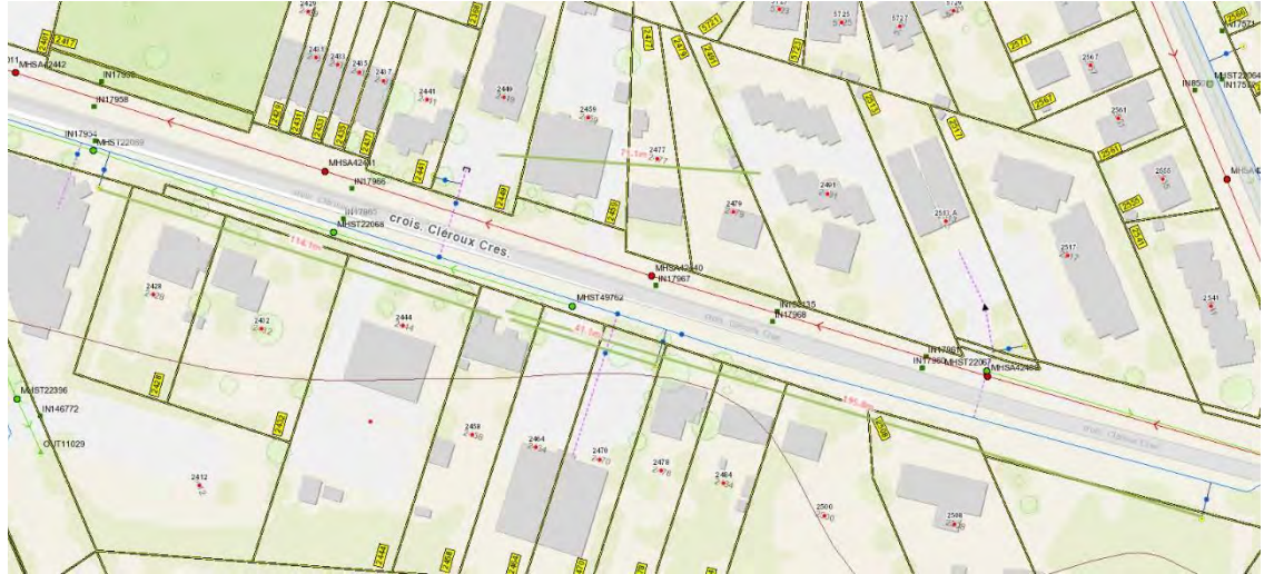
2458 Cleroux Cres, Ottawa: Hydrants location and distance
