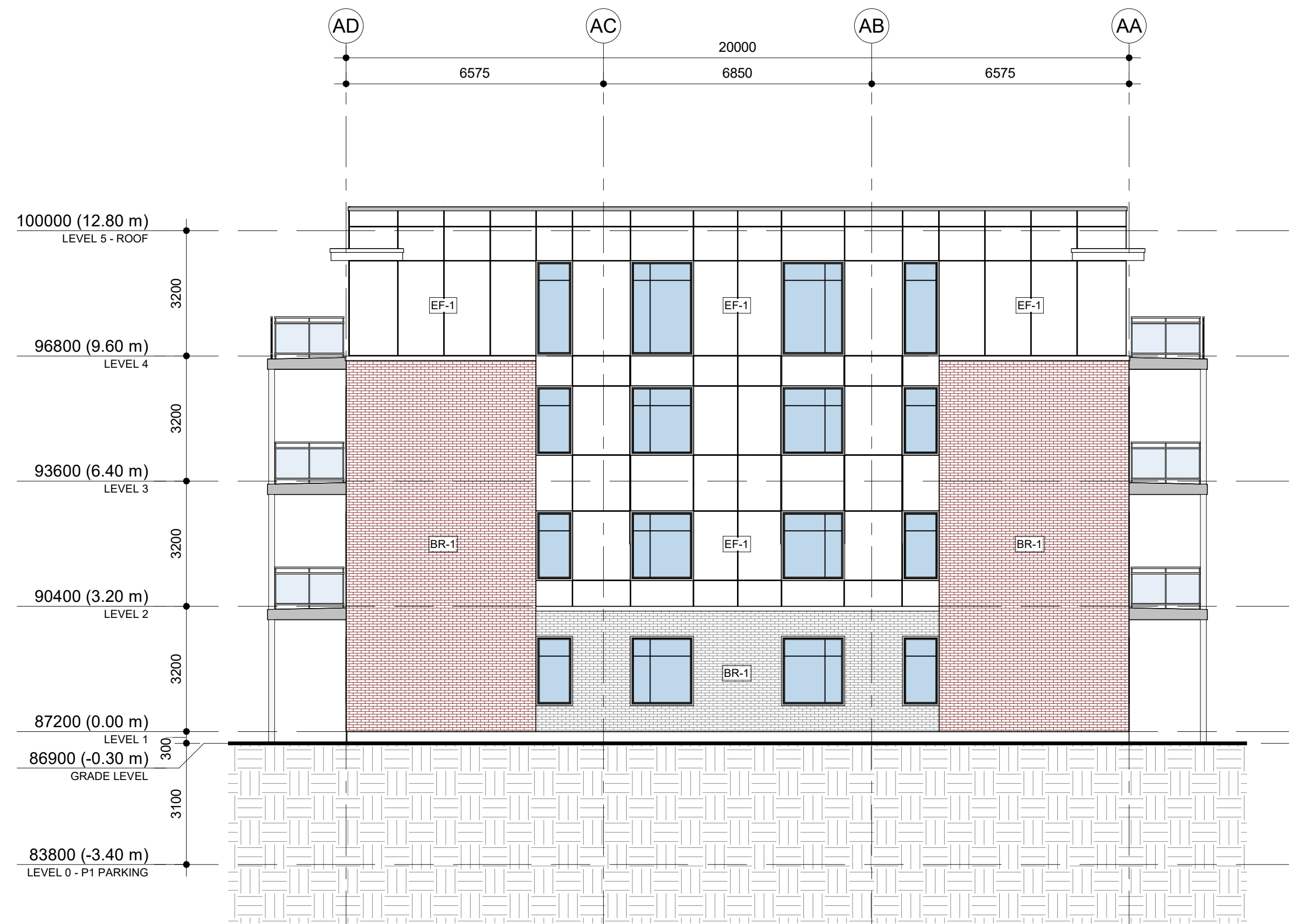
1 BUILDING A - NORTH ELEVATION A201 1 : 100
