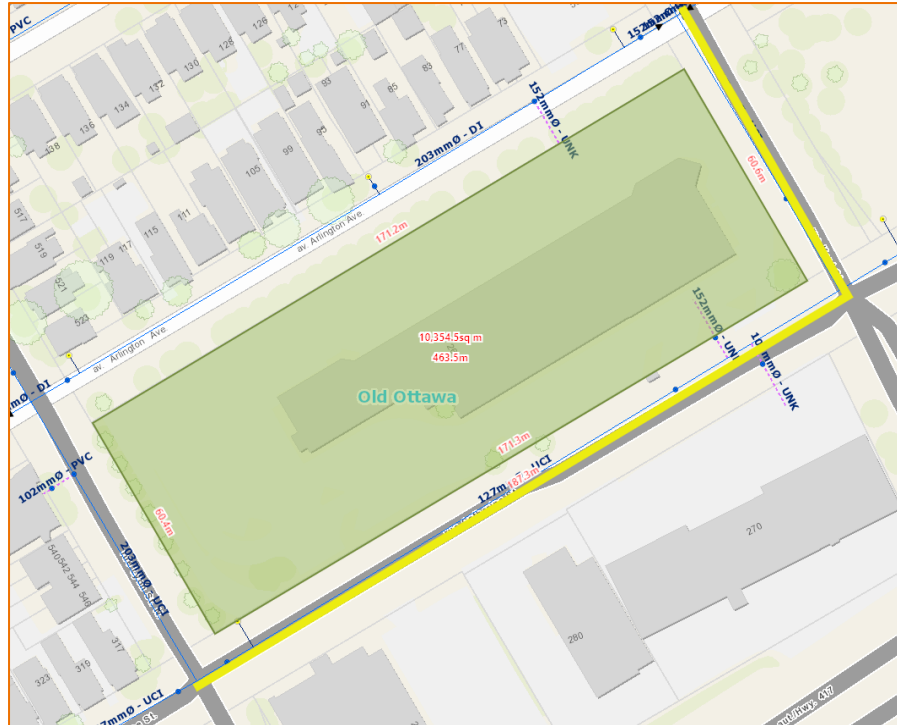
Figure 3.2: Sketch of proposed watermain upsizing in Catherine Street and Kent Street
