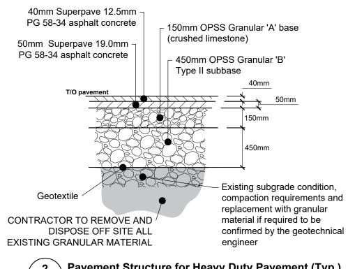
2 \ Pavement Structure for Heavy Duty Pavement (Typ.) C4 / Scale: As shown
