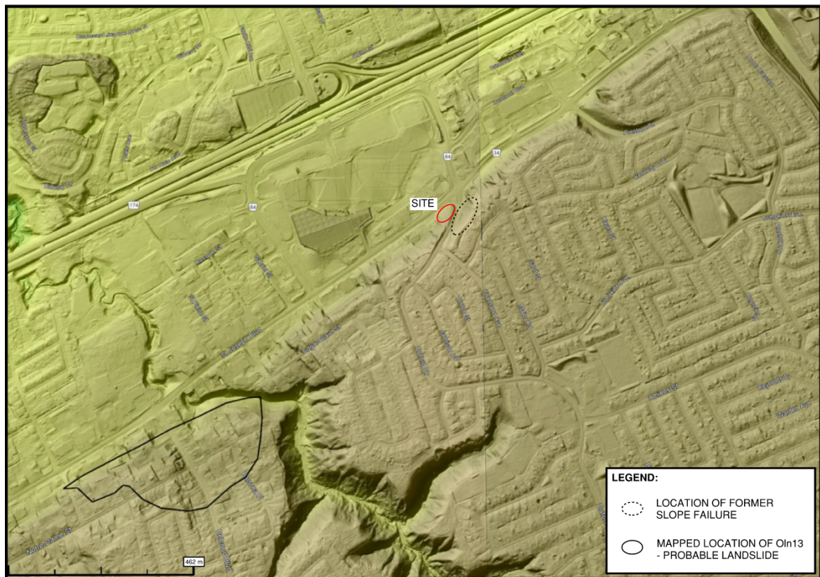
Figure 1 – LiDAR Image of Subject Site and closest landslide and slope failure.
