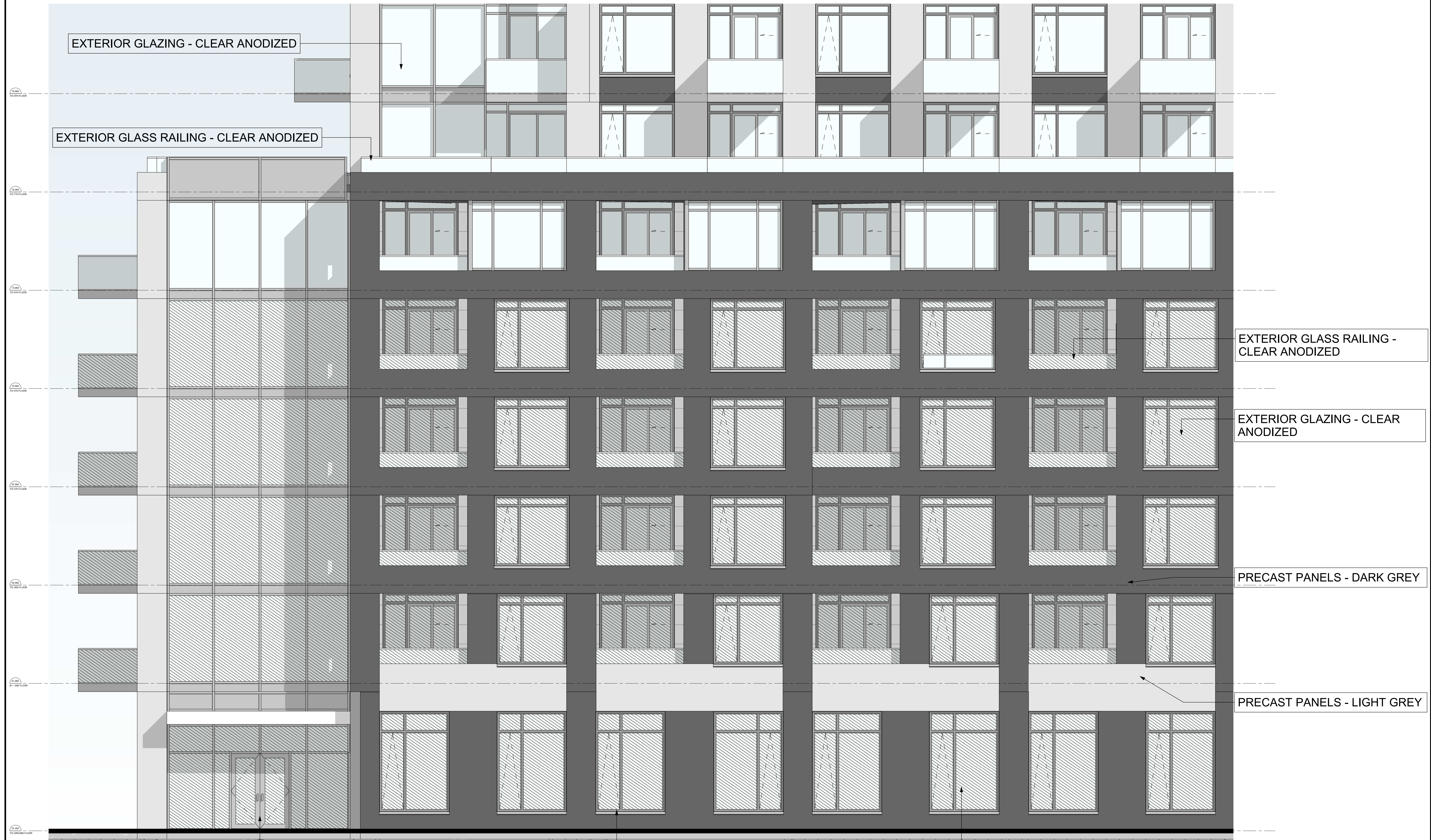
BUILDING B1 - SOUTH ELEVATION
