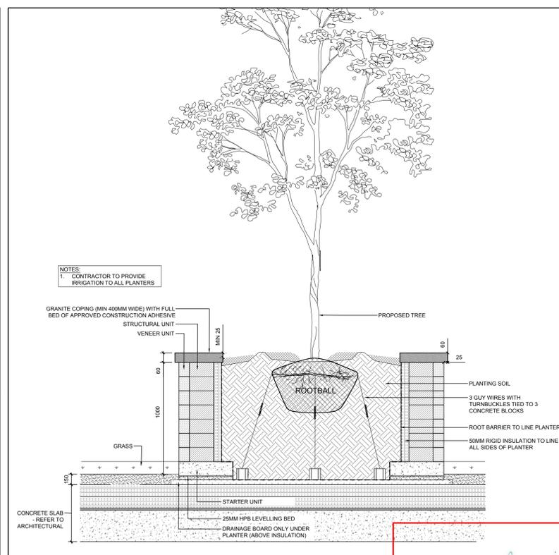
**6 PRECAST CONCRETE PLANTER ON CONCRETE SLAB**
