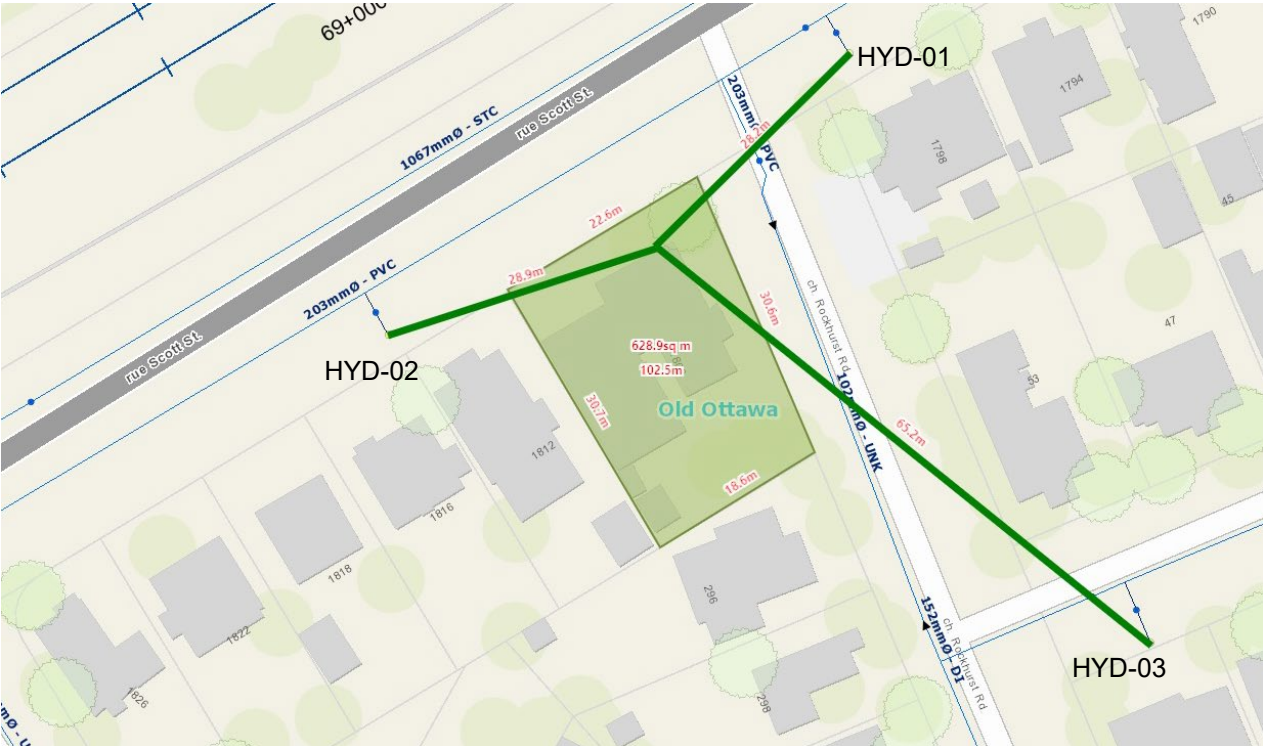
Figure 2: Fire Hydrant Coverage Sketch
