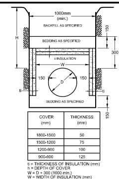
W = D + 300 (1000 min.) W = WIDTH OF INSULATION (mm) D = O.D OF PIPE (mm)
