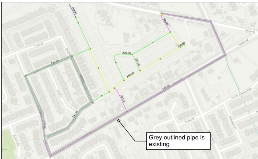
Figure 1 – Proposed Watermain Sizing & Layout
