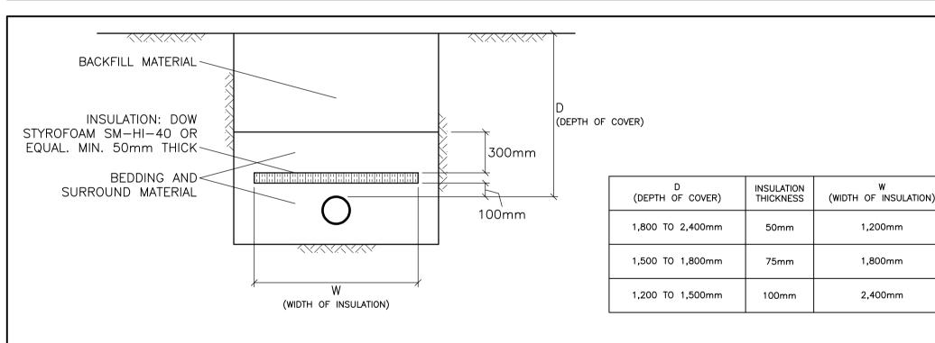
INSULATE WATERMAINS AND WATER SERVICES AS INDICATED AND WHERE DEPTH OF COVER IS LESS THAN 2,400mm.
