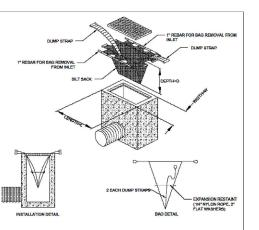
INLET SEDIMENT CONTROL DEVICE
